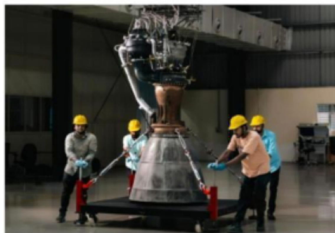
Frontier tech: The Full-Flow Staged Combustion LOX-Methane rocket engine. SPECIAL ARRANGEMENT
